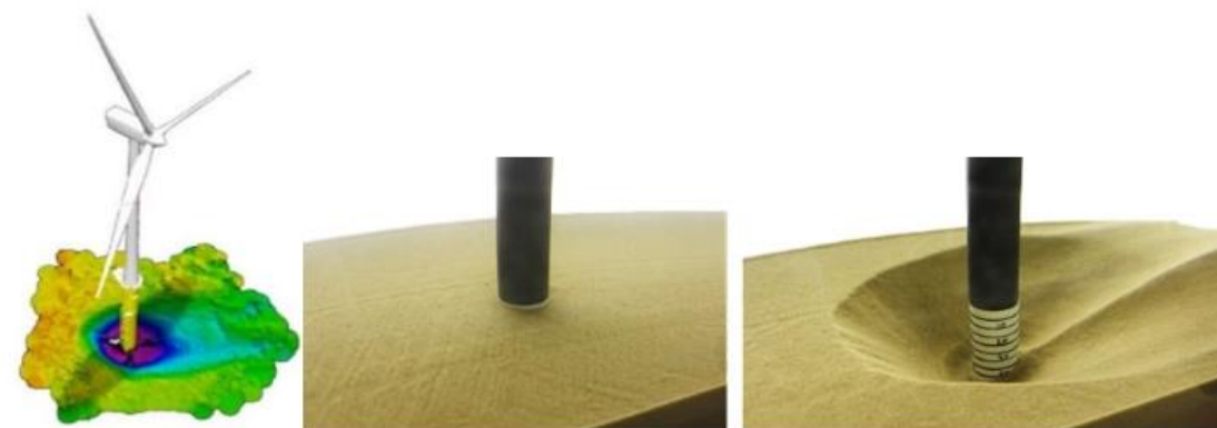
Figure 12. Scour development around a monopile foundation (illustrations: EIWA).
