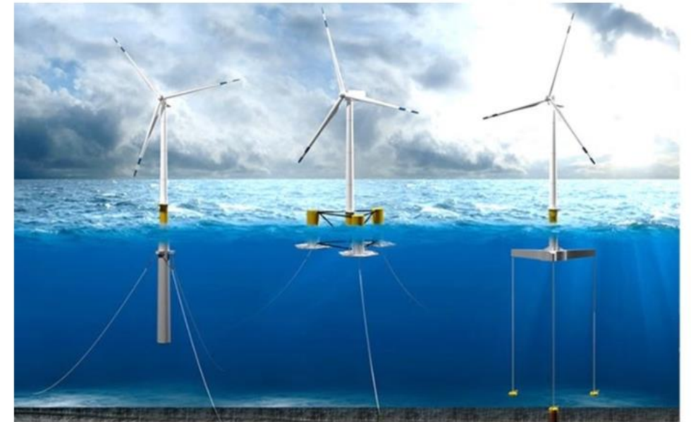
Figure 23. From left to right: SPAR, Semisub and TLP type of OWT floaters (Illustration: DNV-GL).
